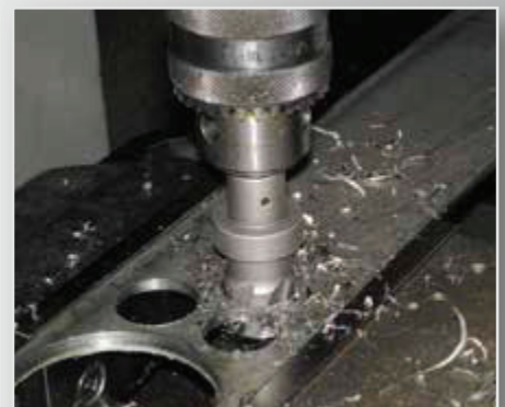
Drilling flat steels
